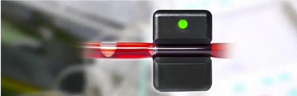
In the medical industry, there is always a need for new and innovative technologies that can help improve patient care. Bubble detectors are one example of how technology is being used to make a difference. A [bubble sensor](#) is a small device used to detect the presence of bubbles in fluids. They are placed inside intravenous (IV) bags and work with sensors to identify the presence of air bubbles in the IV solution.
